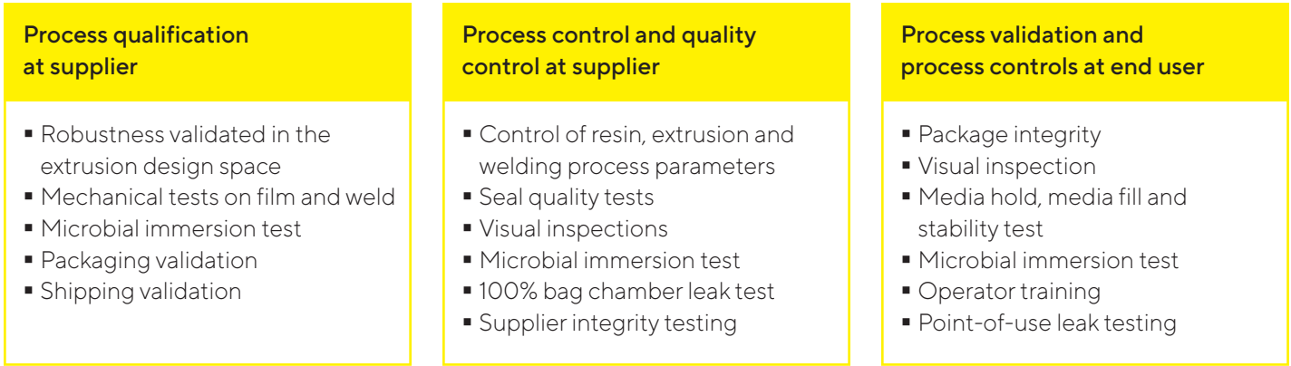
Figure 9: Assurance of Flexboy® container closure integrity along the entire life cycle
